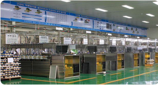
Electronic automatic water meter testbench 1,6 (Metrological Class horizontal R100 to R200) (15 to 50mm)
