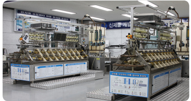
Electronic automatic water meter testbench 1,6 (Metrological Class horizontal R100 to R200) (15 to 50mm)
